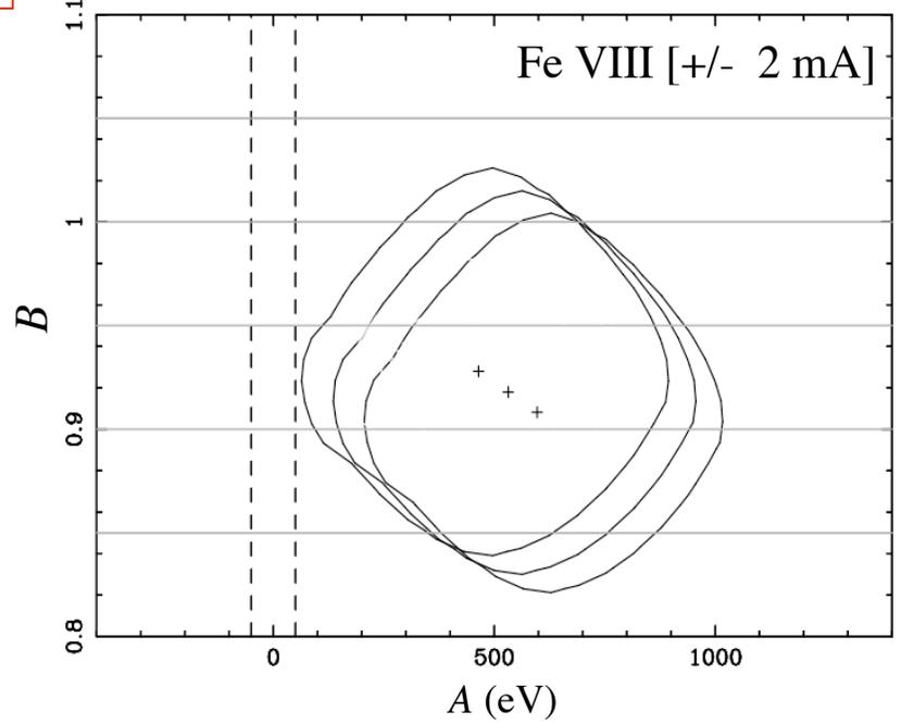
*Unprecedented precision in constraining the ionization state of Fe responsible for the narrow XIS Fe K line due to the redundant information provided by the high SNR Fe K $\beta$  line. States higher than Fe VII are ruled out after conservatively accounting for instrumental and theoretical uncertainties.*
