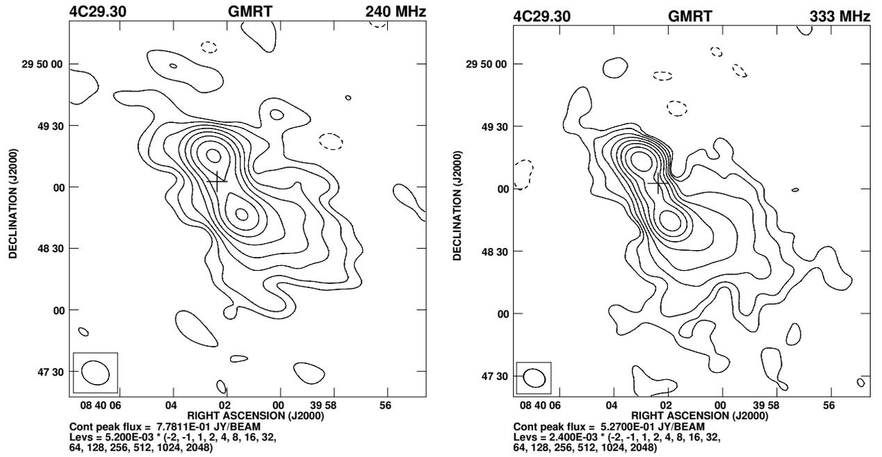
Figure 10: The GMRT images of 4C29.30. Left panel: Image at 240 MHz with an angular resolution of  $13.8 \times 11.1$  arcsec<sup>2</sup> along PA 64°; right panel: the 334-MHz image with an angular resolution of  $10.6 \times 8.5$  arcsec<sup>2</sup> along PA 68°.
